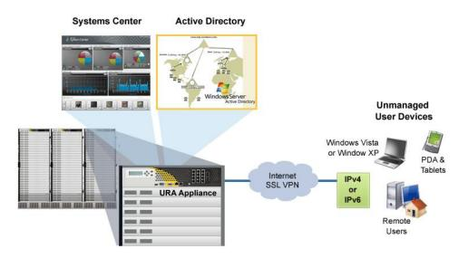
UAG 2010 provides endpoint protection and interrogation, where an end user computer must pass the corporate access policies before access is allowed. This provides an easy to use remote access solution through a web browser, all enabled on top of the Windows Server 2012 platform.
