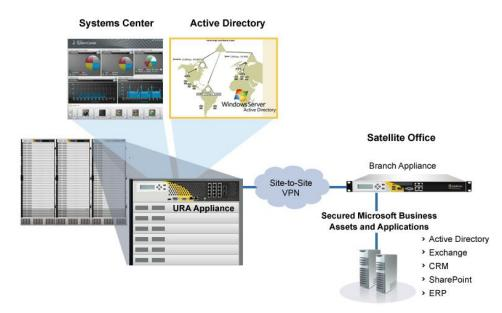
The Site-to-Site VPN links corporate sites and are commonly deployed as WAN backbone links. When combined with routing protocols, VPN circuits can be deployed in mesh networks.
